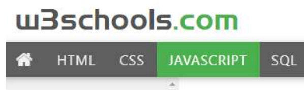
Fig 65: Example of a navigation bar using 'active' page indication, by highlighting the current page in a different colour to that used for the rest of the bar
